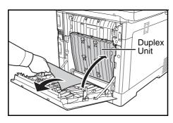
6 If a paper jam reaches the Duplex Unit as shown, lift up the Duplex Unit and remove the paper.
